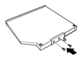
Figure 4-29 Removing ODD bracket
